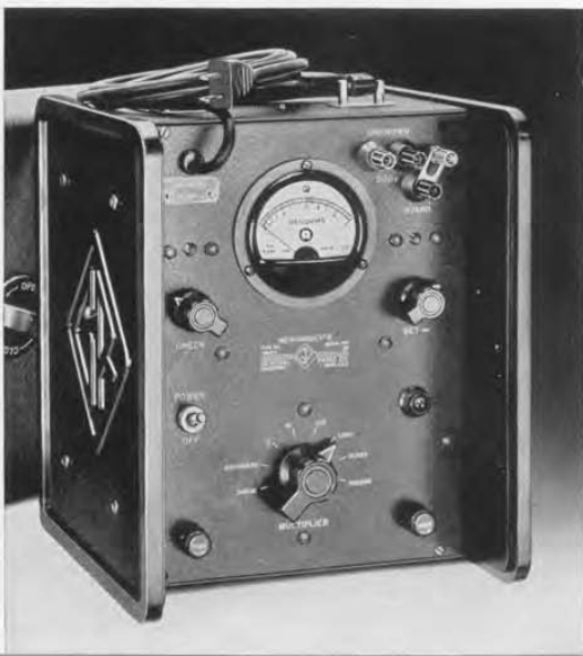
Figure 1. View of the megohmmeter with cover removed to show panel.
